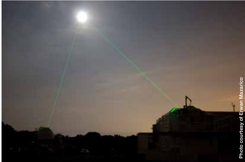
LOLA's range imaging system can optically detect laser pulses from Earth, determining LRO's precise orbit position
